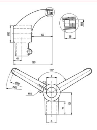
d (inch) = 1 1/2 Gas d1 (inch) = 1 1/2 Gas d1 (mm) = 48.3 d mm = 48.3 Weight (g) = 720
